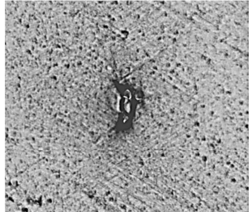
Slip-line detection in 200 mm Silicon
