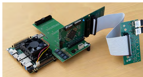
FPGA master control unit with redundant optical Gbit interface to MMC cells with transmission times as low as 2 μs © Christian Braschwitz / Fraunhofer IISB
