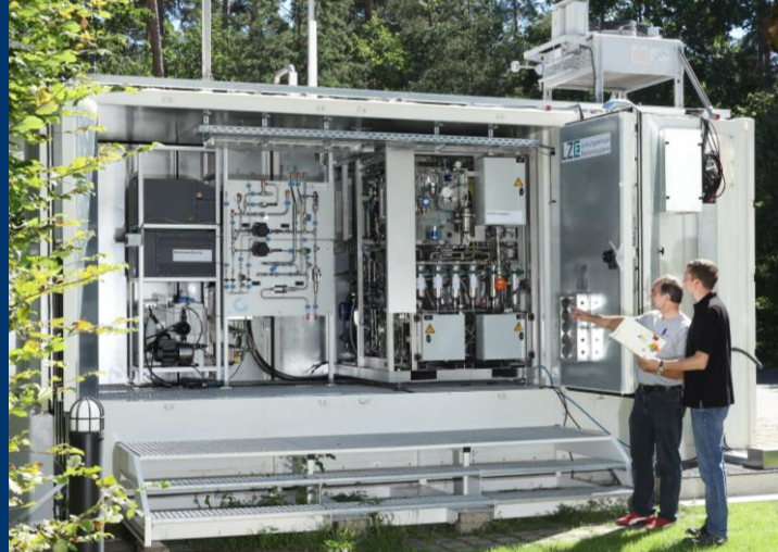
Test bench: 1 MWh LOHC storage system
